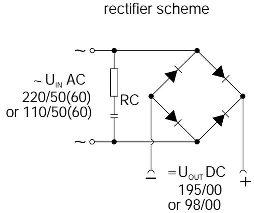
AC and DC solenoids have the same dimensions , connections and characteristics. The difference between AC and DC solenoids is in the integrated rectifier into the AC type - see "rectifier scheme". The solenoids can be used for 50Hz and 60Hz. The supply voltages are as follows: 12V DC , 24V DC , 48V DC , 110V AC/50(60)Hz and 220V AC/50(60)Hz.
