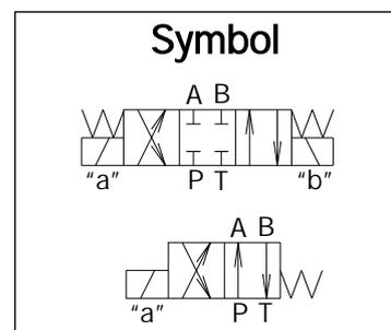
The RH10...1...-...F... valves are solenoid operated directional spool valves. They are control the start , stop and direction of flow.
